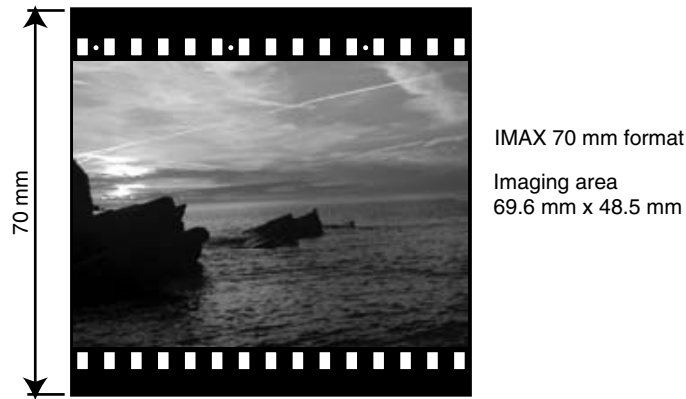
Figure 4-6 IMAX film dimensions.
