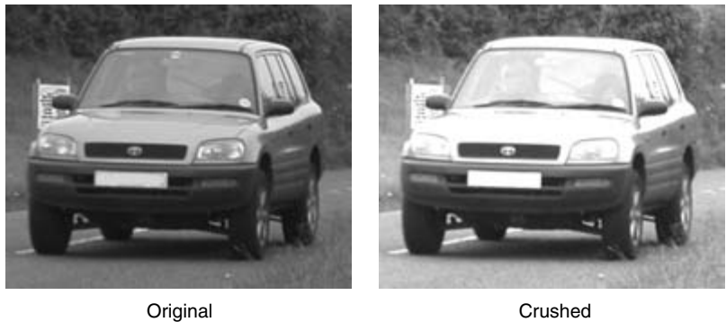
Figure 6-17 Crushing effect when white values exceed peak.
