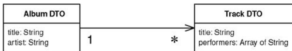
Figure 15.6. A class diagram of data transfer objects.
