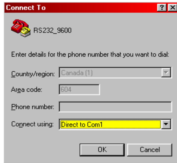
Fig F69 HyperTerminal: connection port selection
