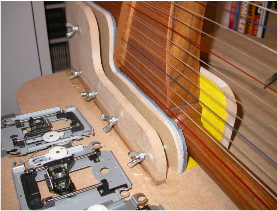
Figure 6-3. The harp's clamping arrangement
