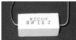
Figure 3-5: A 5-watt resistor
