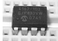
Figure 17-11: Microchip Technology's MCP4162 digital rheostat
