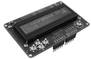
Figure 13-6: The Freetronics LCD & Keypad shield
