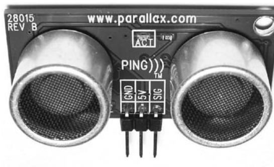
Figure 12-26: The Ping))) ultrasonic distance sensor
