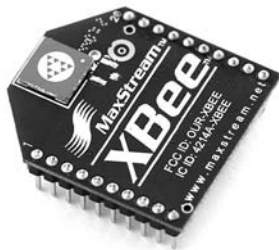
Figure 14-6: Typical XBee transceiver
