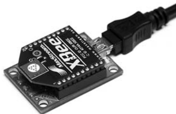
Figure 14-8: XBee connected via USB with an Explorer board
