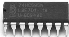
Figure 6-4: The 74HC595 shift register IC
