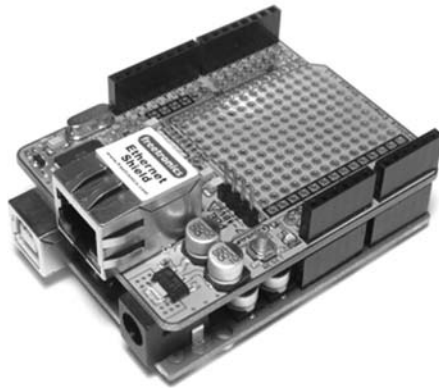
Figure 8-1: Ethernet shield on Arduino Uno
