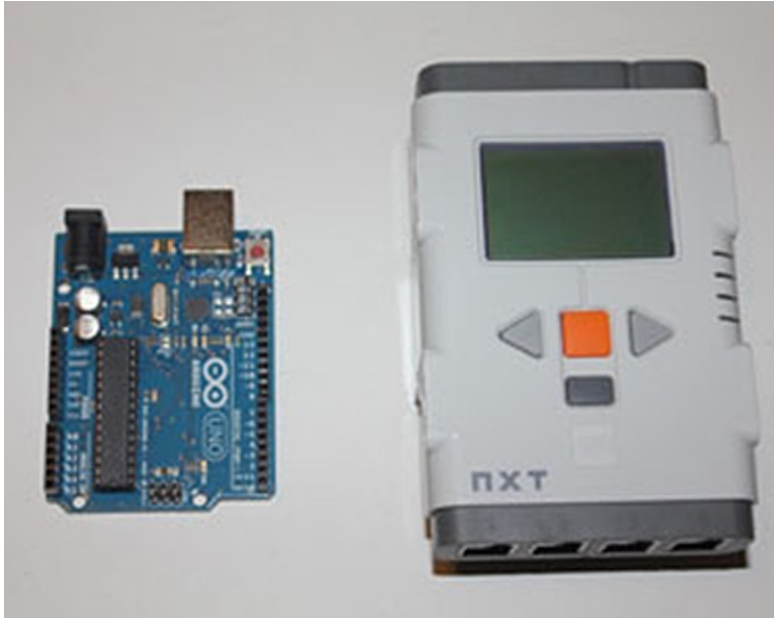
Figure 1-2. The Arduino and the LEGO Mindstorms NXT Intelligent Brick
