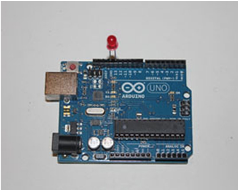
Figure 1-4. The LED plugged into the Arduino
