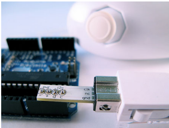
Figure 9.6 WiiChuck designed by Tod E. Kurt
