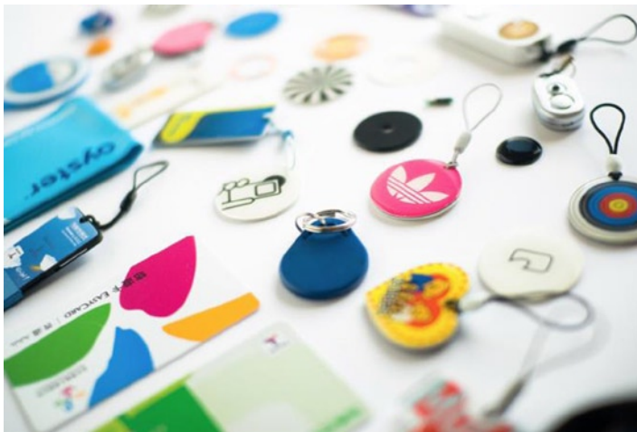
Figure 16-2. RFID tags and cards come in all shapes and sizes (image courtesy of Timo Arnall)
