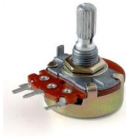
Figure 3-3. A rotary potentiometer (image courtesy of Iain Fergusson)
