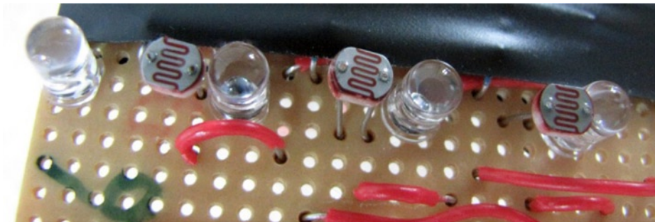
Figure 10-10. The sensor bar consisting of four LEDs and three LDRs
