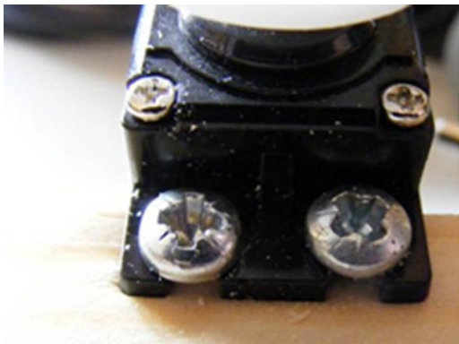
Figure 4-6. Using self-tapping cheesehead screws
