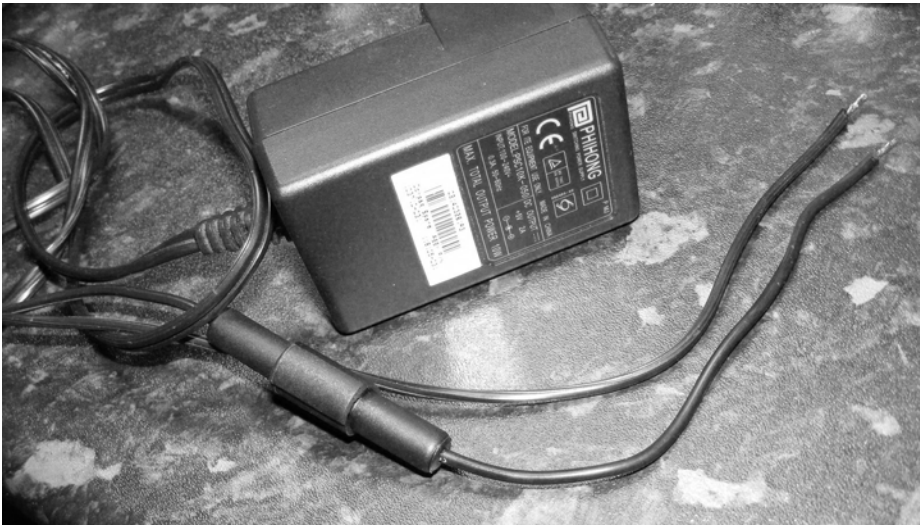
Figure 2-5. A repurposed 5 volt supply
