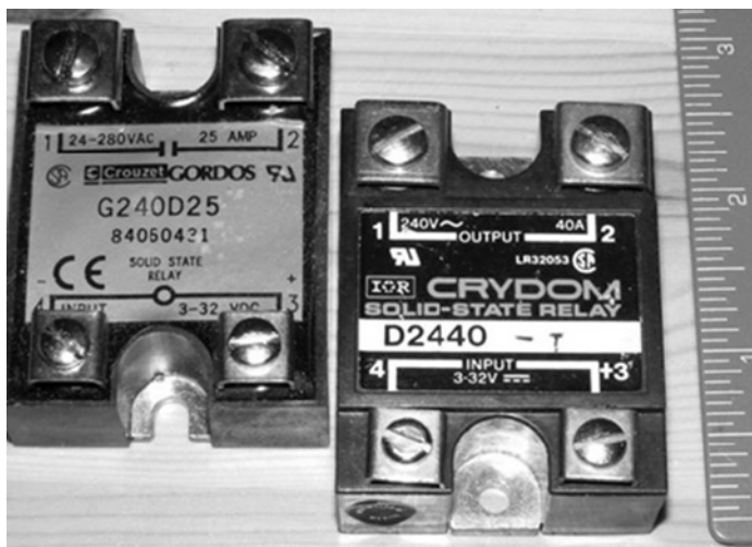
Figure 4-26. Two examples of a solid state relay
