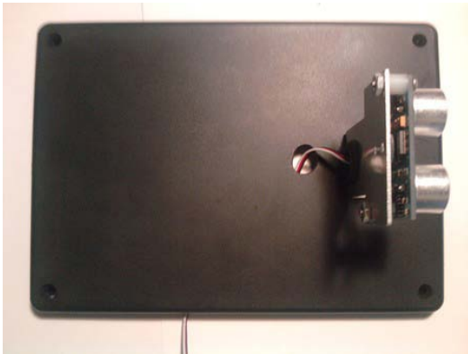
Figure 8-6. Attach ultrasonic sensor to bracket.
