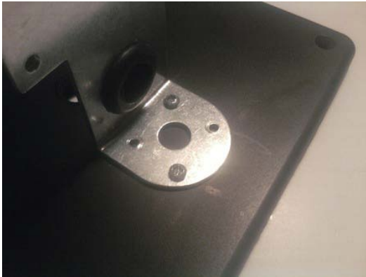
Figure 8-5. Connect ultrasonic bracket to lid of the enclosure.
