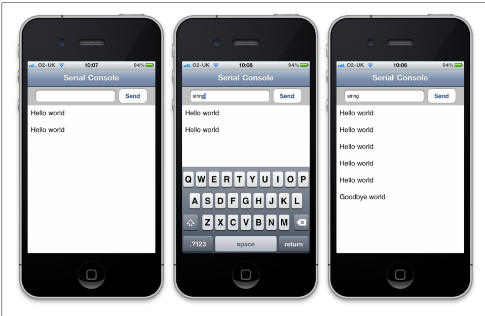
Figure 2-16. Application connected to the Arduino (left), entering characters (middle), which have been received by the Arduino (right)
