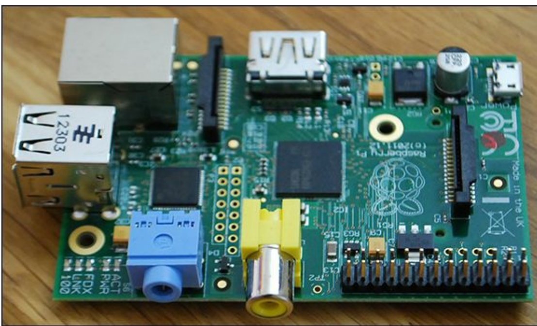
Figure 1 The Model B revision of the Raspberry Pi, about the size of a credit card
