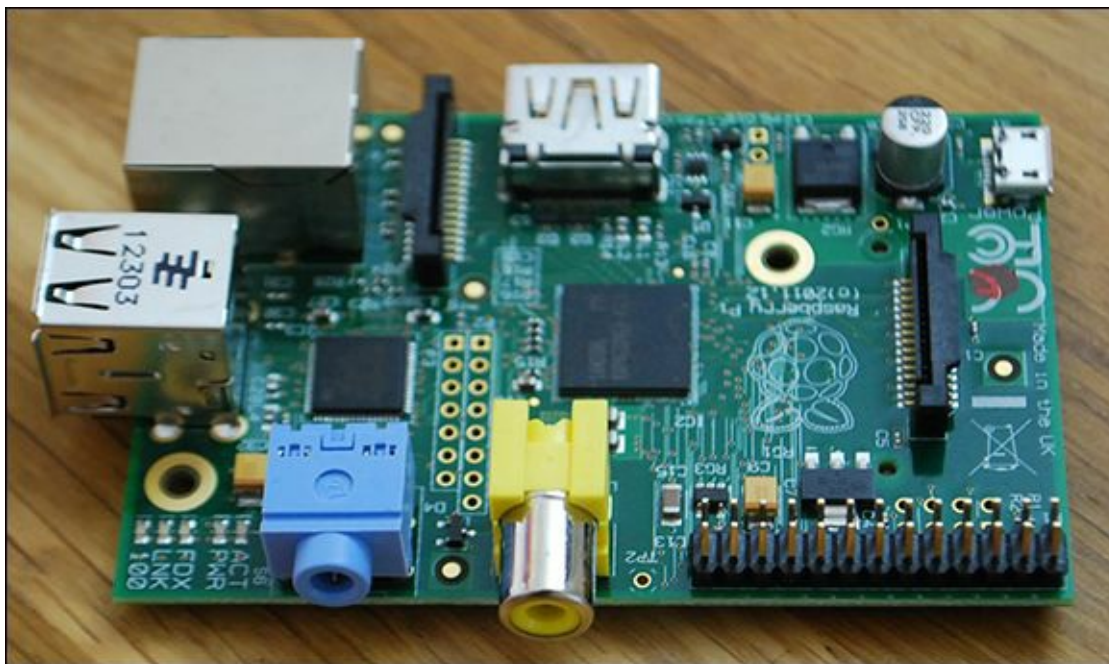
Figure 8-1 The General Purpose Input Output (GPIO) pins on a Model B Raspberry Pi
