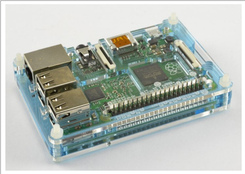
Figure 1-2. A Raspberry Pi 2 in a PiBow Coupé
