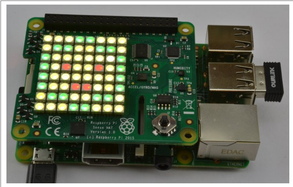
Figure 14-3. A Sense HAT displaying an “image”
