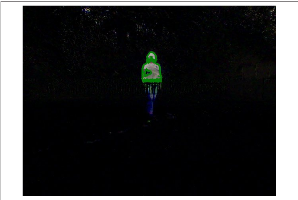
Figure 8-9. Movement detection blobs
