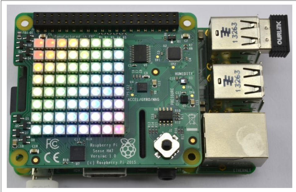
Figure 9-19. The Raspberry Pi Sense HAT
