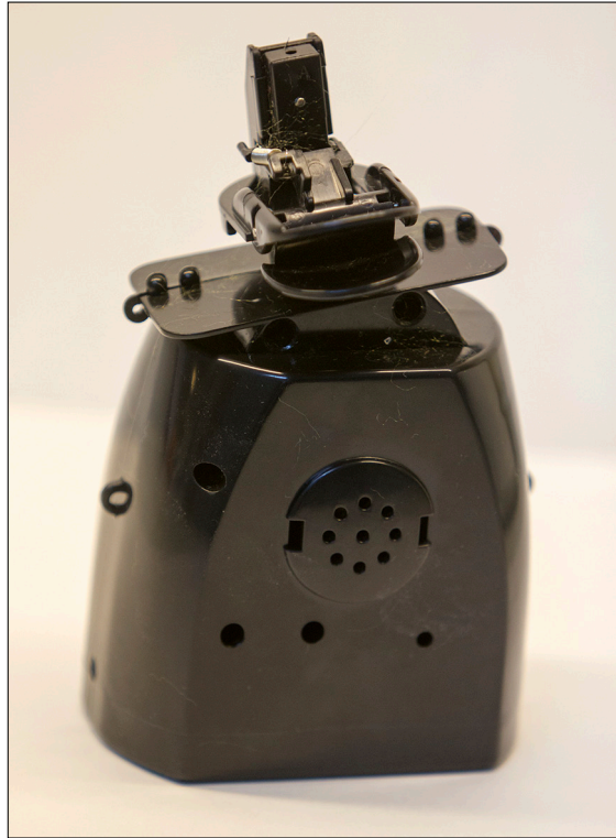
FIGURE 2-1: A naked chicken – the mechanism that makes the toy move.
