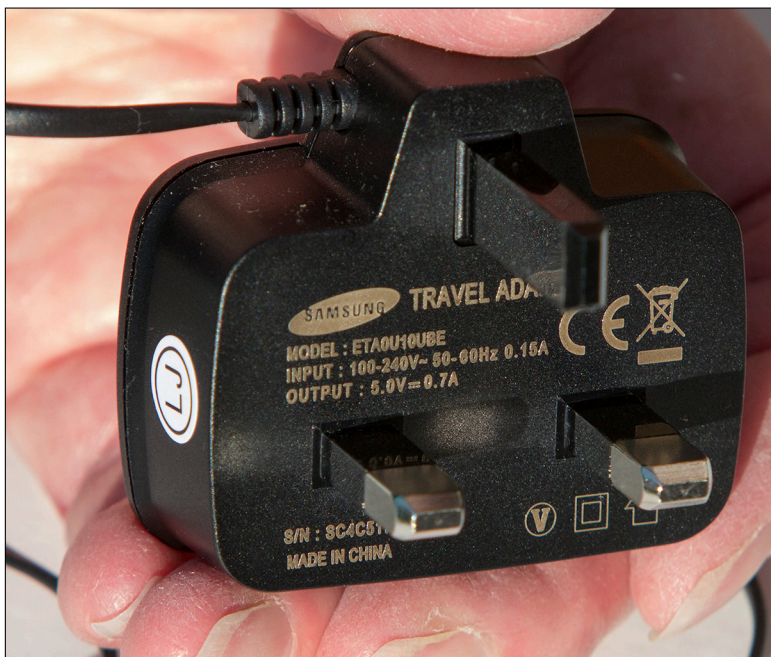
FIGURE A-13: A power supply showing its output rating.
