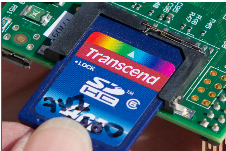
FIGURE A-11: Take care not to snap off the plastic that keeps the SD card from falling out.
