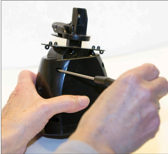
FIGURE 2-2: Removing the case of the movement mechanism.
