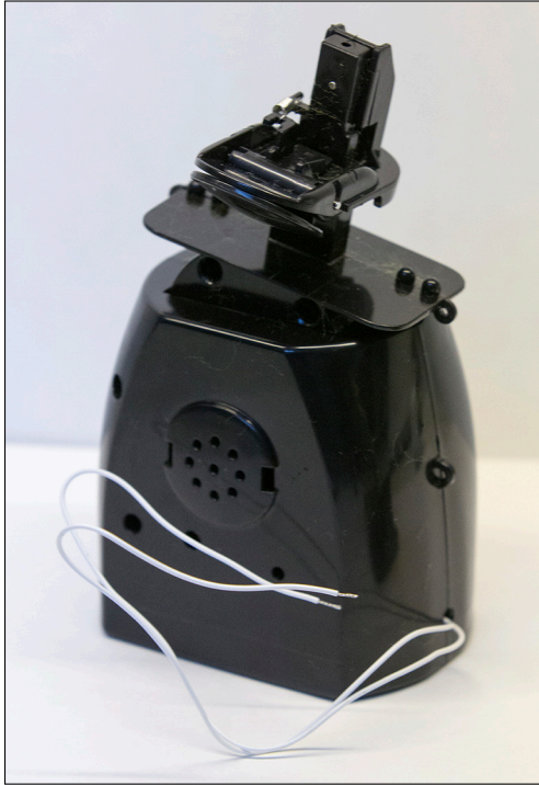
FIGURE 2-4: Toy post-surgery showing no ill effects. Touch the wires together to make the toy move.
