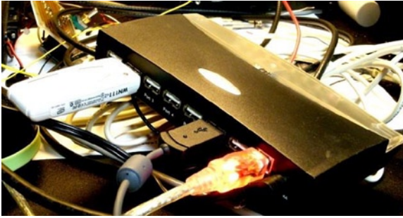
Figure 6-2. A powered USB hub
