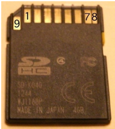
Figure 8-1. SD card pinout
