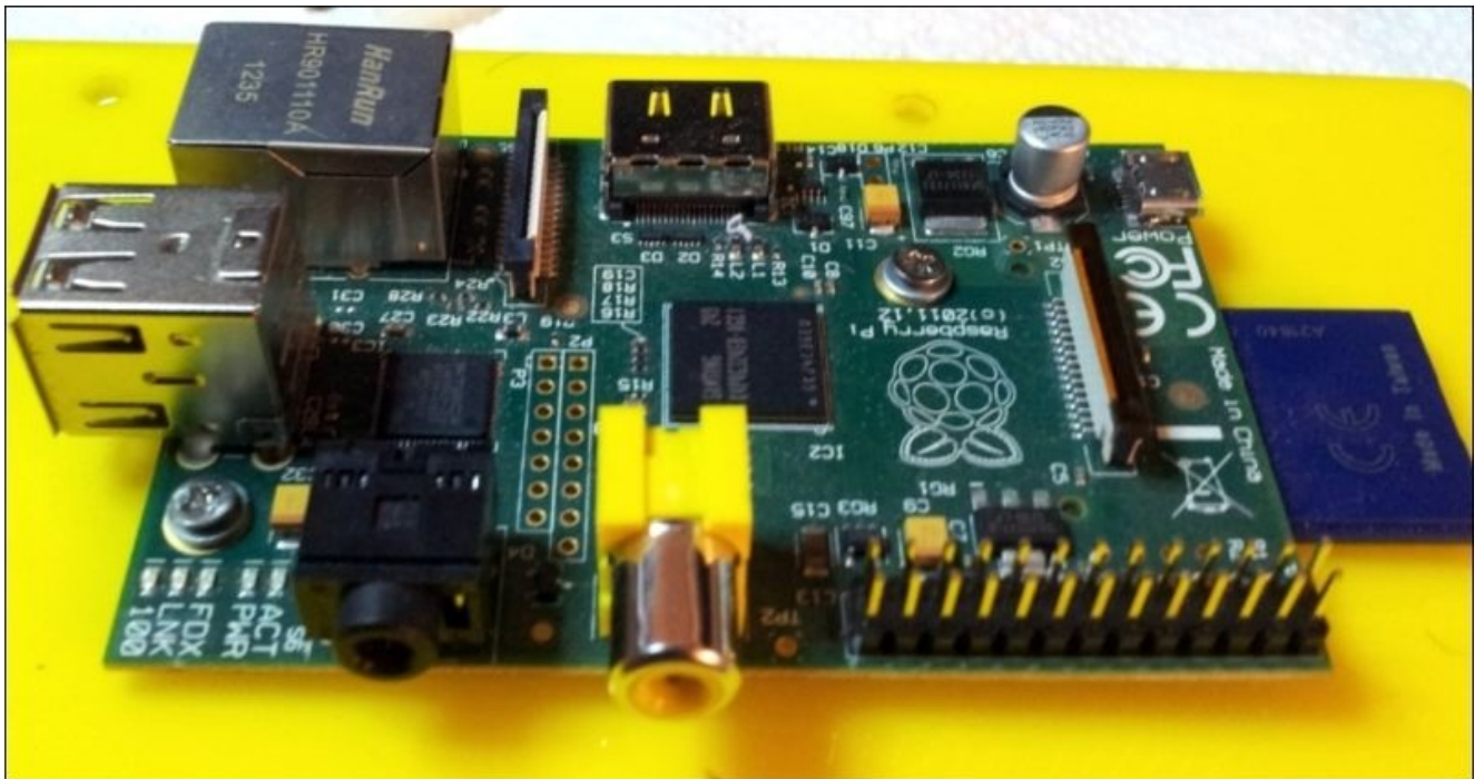
Raspberry Pi mounted using M2.5 screws
