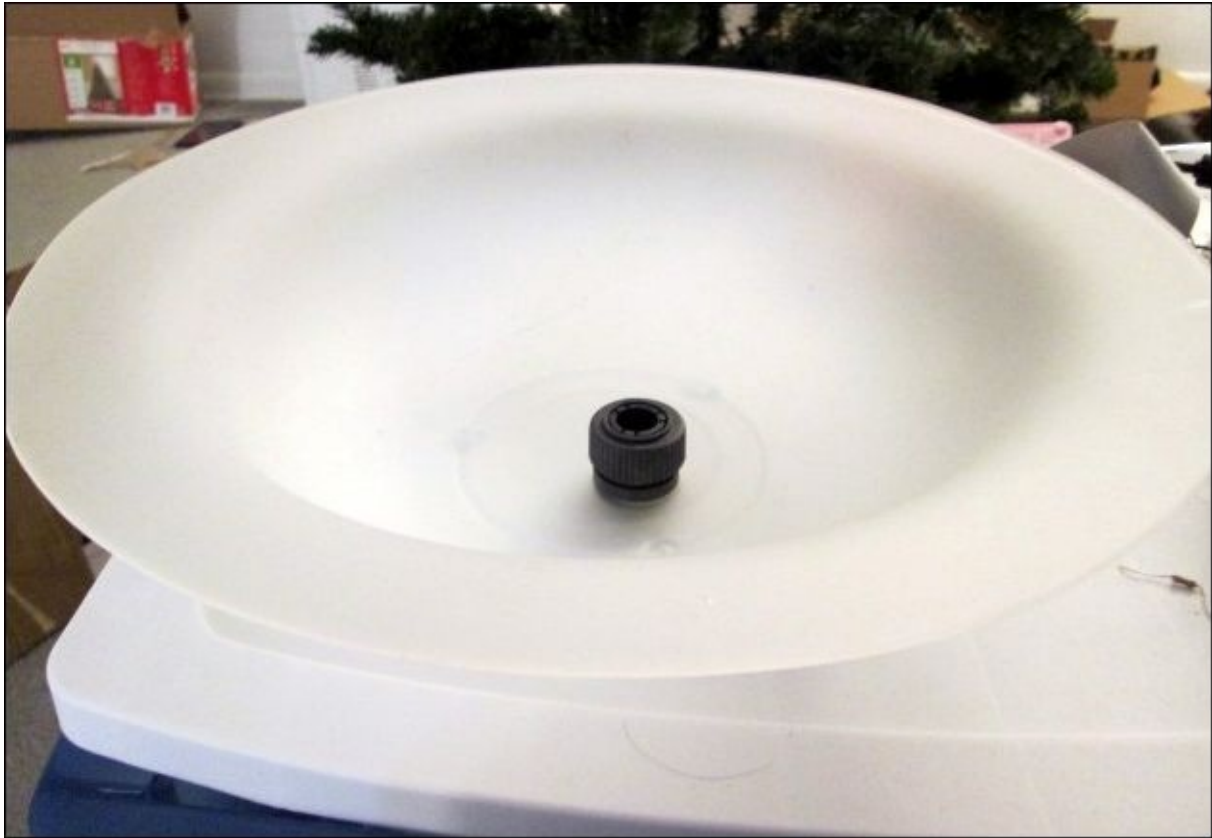
A basin with a sealed electrical outlet
