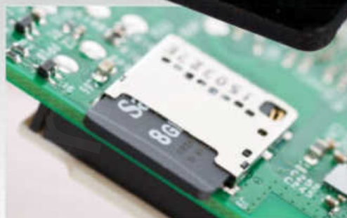
Left Among the minor changes is a return to the old slide-lock microSD card slot – no more push-to-eject
