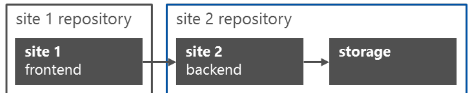
Figure 2: Splitting an application into independent deployable components
