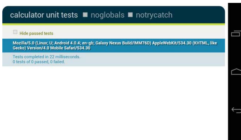
Figure 9-2. Running QUnit tests in the browser
