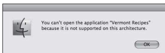
FIGURE 8.19 An alert warning that the unmodified application cannot be run on a PowerPC Mac.
