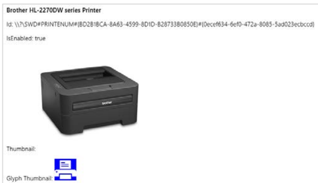
FIGURE 15-4 Sample device enumeration output for a printer—which also looks exactly like the one sitting next to my desk.
