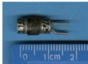
FIGURE 1.7 A transistor, which replaced the vacuum tube
