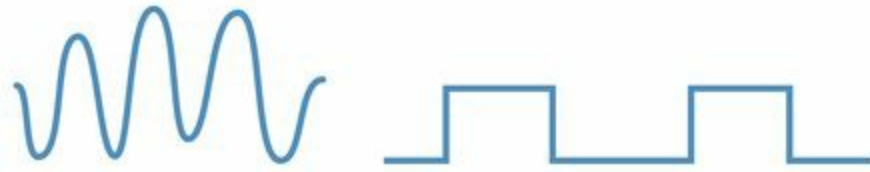
FIGURE 3.2 An analog signal and a digital signal
