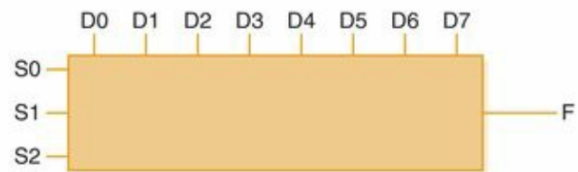
FIGURE 4.11 A block diagram of a multiplexer with three select control lines
