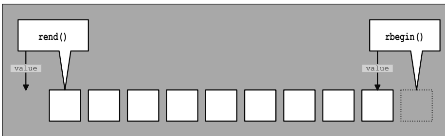
Figure 9.3. Position and Value of Reverse Iterators
