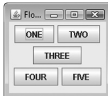
FIGURE 14-10. Component placements in FlowLayout after window resizing
