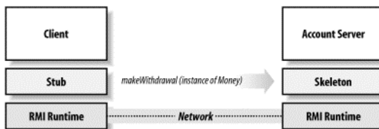
Figure 10-1. Runtime structure when making a withdrawal
