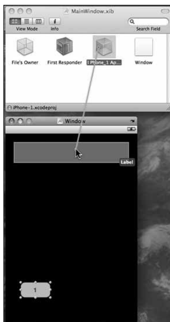
Figure 21.18 Connecting an outlet variable.
