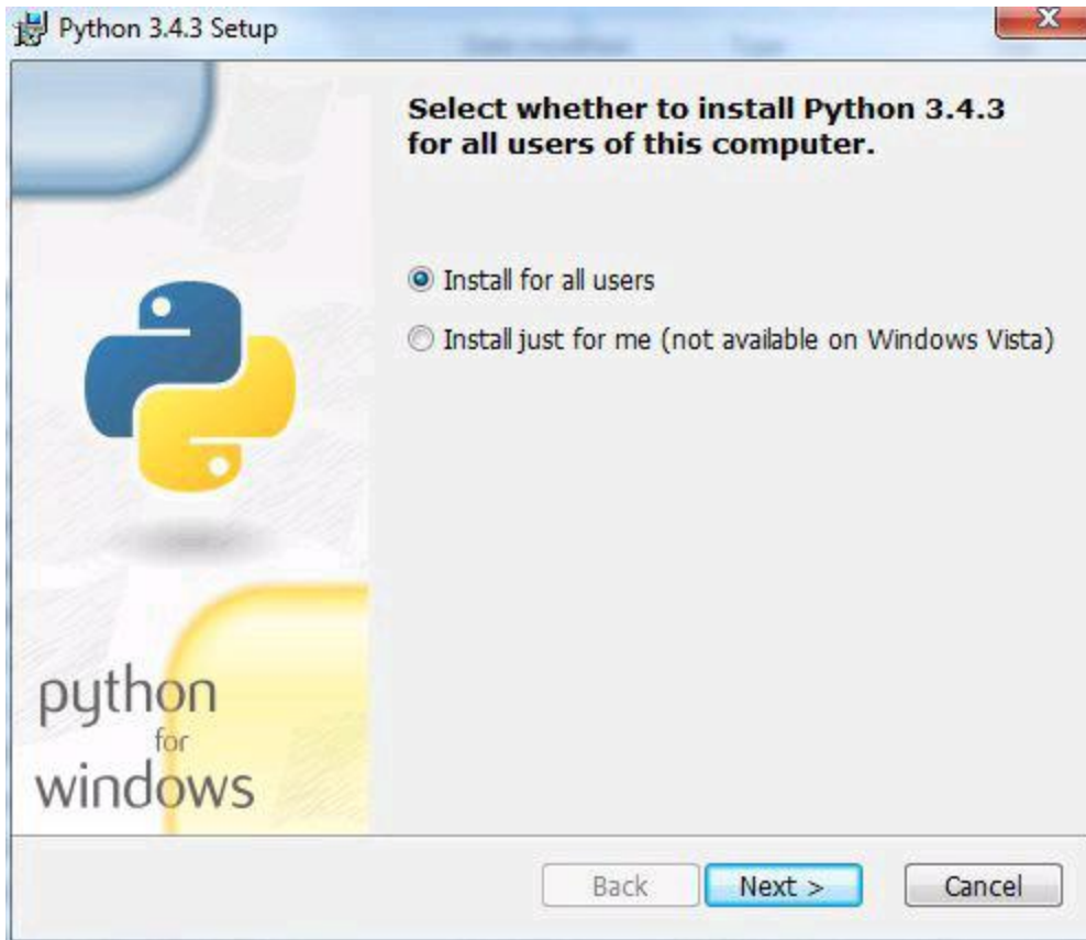
Figure 3: Screenshot of the Python installation process A good practice is to enable the option to run Python from your command line. To be able to do that, you should select Entire feature will be selected on local drive in the Customize Python 3.4.3 window as showing in the following picture.
