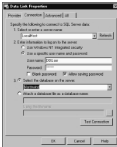
Figure 9.2 Connection Options for a SQL Server OLE DB Provider
