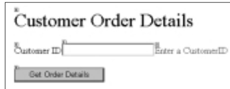
Figure 10.8 RequiredField Validation Control in Design Time
