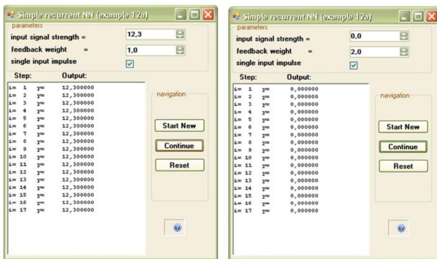
Figure 11.4 Two ways of achieving state of equilibrium in a linear network: zero signals (left) or single feedback amplification without simultaneous input signal (right).
