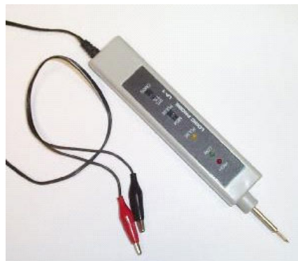
Figure 10. An example of a digital logic probe
