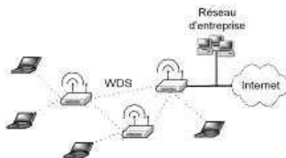
Figure 3.16 — Le Wireless Distribution System (WDS).
