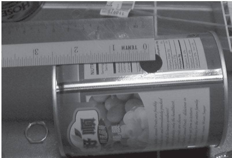
Figure 8-7 Measure and drill hole for antenna connector (photo courtesy of Julian “HammerJammer” Ho).
