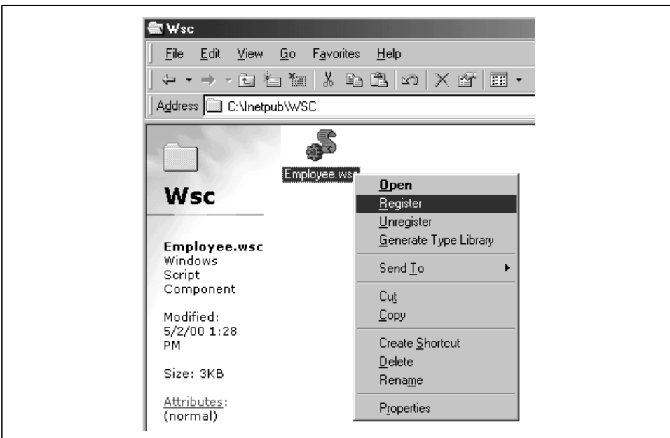
Figure 7-11. To register a Windows Script Component, right-click the .wsc file and choose Register
