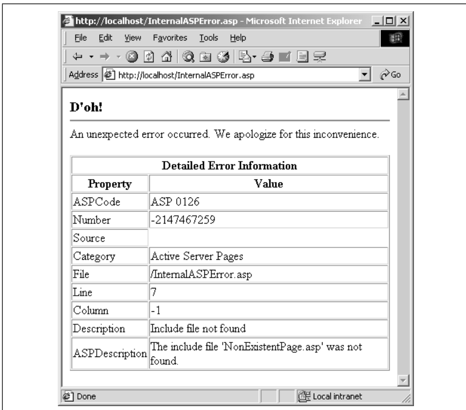
Figure 3-6. An internal ASP error produces these values in the ASPError object's properties
