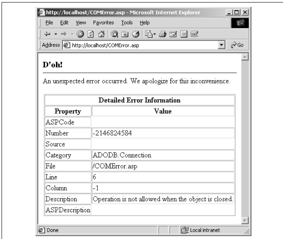
Figure 3-7. An external COM object error produces these values in the ASPError object's properties
